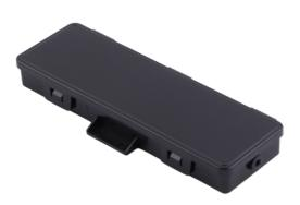
The fiber optic splice closure shell is sealed with EPDM sealing strips, and the optical cable inlet and outlet holes are sealed with silicone sealing rings. The head shell is sealed with buckles, which makes opening and installation more convenient, construction is faster, and the sealing performance of the product is better.
