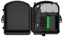
The fiber distribution box shell is made of modified PC +ABS material, and the internal metal parts are made of high-quality steel plate materials. It can meet the service life of more than 20 years (depending on the environment), and has good impact resistance and resistance. Corrosion properties.
