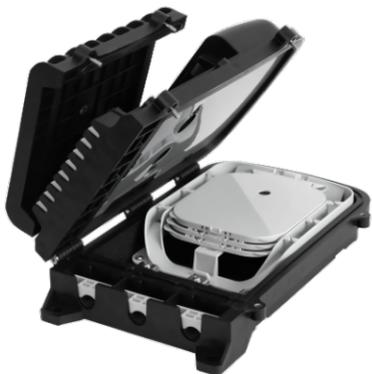
Optical fiber splicing trays and storage tray adopt a friendly modular structure design. The number of splicing trays can be increased or reduced according to capacity to meet the needs of different users. Supports coiled storage of optical fibers with loose tubes, and the bending radius of the optical fiber is greater than 30 mm.
